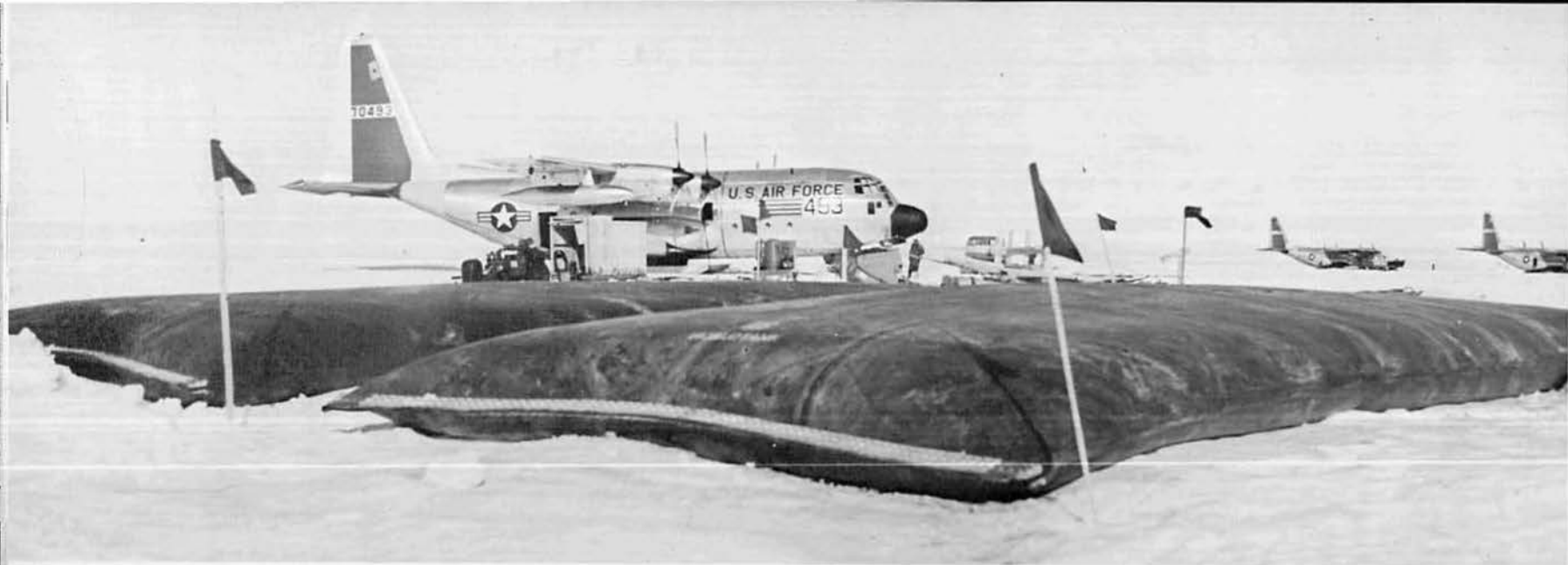
10,000 gallon combat fuel cells were used to quench the thirst of the huge C-130's.
