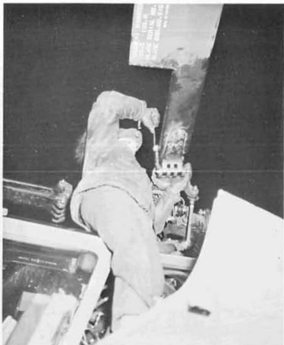
As the "Choppers" are pulled out of the hangar, the rotors are bolted in place (above), and checked for alignment (below).
