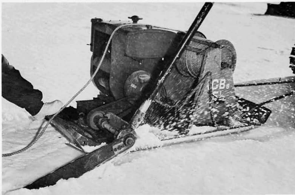
The ice saw is used to cut a berth for the USS ARNEB.
