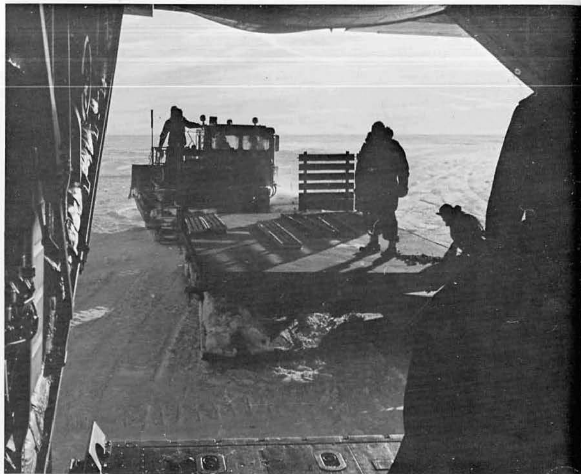
Backing a 20 ton sled up to the cargo hatch of a C-130.
